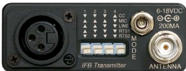
The IFBT4 rear panel provides the audio input and programming DIP switches for intercom and audio input type along with power and antenna input jacks.
